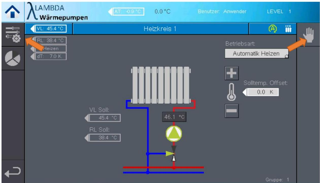
The screenshot shows the LAMBDA control interface for 'Heizkreis 1'. The top bar displays 'AT: -0.9 °C' and '0.0 °C'. The left sidebar shows 'VL: 45.4 °C', 'RL: 38.4 °C', and 'dT: 7.0 K'. The main area features a heating circuit diagram with a radiator and a pump. A temperature sensor is shown with a reading of '46.1 °C'. On the right, the 'Betriebsart' is set to 'Automatik Heizen', and the 'Solltemp. Offset' is '0.0 K'. A hand icon in the top right corner indicates a manual test function.
