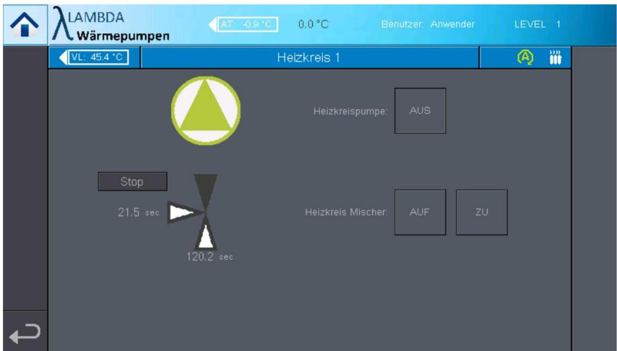
The screenshot shows the manual control options for 'Heizkreis 1'. The 'Heizkreispumpe' is currently 'AUS'. The 'Heizkreis Mischer' has 'AUF' and 'ZU' buttons. A 'Stop' button is also visible. The interface includes a large green triangle icon and a valve symbol with '21.5 sec' and '120.2 sec' labels.
